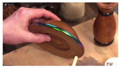
Decoration was done on the three beads with a base of Gesso and a covering of chameleon flecks applied with a dry lightly loaded brush. Gesso is required for the light colour of the wood and should be allowed 10mins to dry before the flakes are added.
