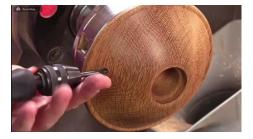
Slight splitting of fibres at the drill entry point was cleaned up with a carving tool. The piece was sanded and finished.
