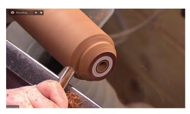
With a careful look at the grain etc of the piece of wood, she decided which way round it would look best when finished. She then mounted it in the chuck by the tenon which would become the base of the piece. With a 1/4in bowl gouge and a 3/8<sup>th</sup> spindle, a concave recess for the 100 mm diameter glass bowl was cut in the end of the piece, ensuring it was a loose fit. The rest of the wood spindle was then shaped including a bead at the bottom of the piece to match that at the top.
