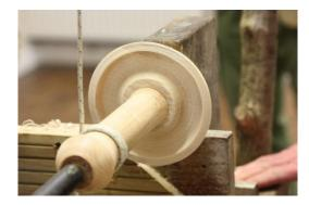
Mike then sat on a chair and carved out the base of the core and tidied up the base of the bowl with a curved double-edged knife moving it towards his hand. These knives were expensive but lasted for ever. After 10 minutes with the knife the bowl was finished.
