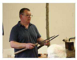
He only used two hook chisels (made by a specialist) which he had mounted on basic hazel handles. The chisel had the cutting angle facing either up or down, the down used for quicker removal of wood. As they looked very similar, he had marked them 'up; and 'down'. Using the wrong one
