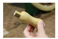
He marked each end of the wood using a three-pronged marker which gave a central indentation and two indentations equally spaced on either side. These he marked as 1,2 and 3 relating them to his diagram to be the centres for his various axes.
