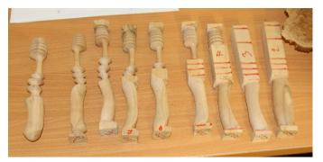
the position on the headstock, the second number emphasised the importance of a very gentle touch and the preservation of the sharp edge transition between coves. Each was sanded lightly before moving onto the next step.
