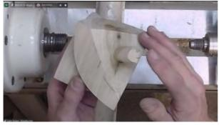
Next a tenon was formed at the tailstock end to enable the piece to be reversed and held in a chuck. That done the hollowing started, checking. the wall thickness at the edges of the bowl before continuing the curve round to remove the wood from the centre portion. Sanding was the next job again observing all the previous precautions.
