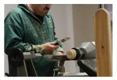
then drill in the centre of the lid being careful not to hit the screw chuck and the lid parted off.
