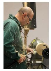
He then shaped the underside of the bowl with his spindle gouge initially using pulling cuts but adding pushing cuts for the final refinement. A flat spot was left at the base. The base was then shear cut with the flat of the gouge with the lathe speed increased to 2000revs. and sanded to 240 grit using a paper
