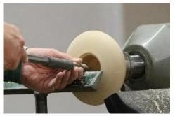
A tenon had been created at the base and the piece reversed in the chuck to allow the top of the bowl to be cleaned up and shaped in a similar way to the base. The size of the lid was then marked out on the
