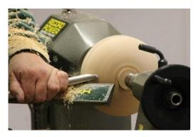
Once the bowl was mounted in his chuck, he marked the surface of the bowl where the final edge would be – about a third of the way from the base.
