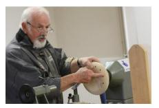
The seat was then remounted on the lathe and the centre hollowed out to make the shape of the seat, and the edges rounded off. Ray emphasized that the edges must be curved not flattened using a twisting motion on the spindle gouge. He sanded it to smoothness.
